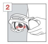
Test the tension of the headband or arm of the defender. Replace if worn.
