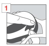
Inspect cushions for any cracks or splits and if worn, replace the cushion.
